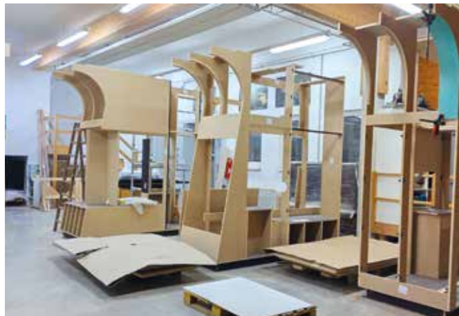
Each individual module had previously been completely assembled and disassembled in the joinery to check the accuracy of fit. Each of the visible panelling panels is glazed several times and then printed by the print shop in a multi-stage process.
