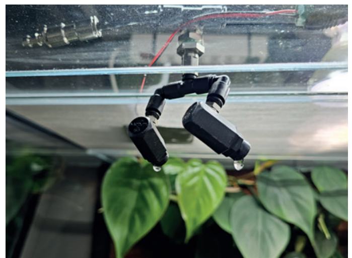
Outlet nozzles of a sprinkler system | Heiko Werning
